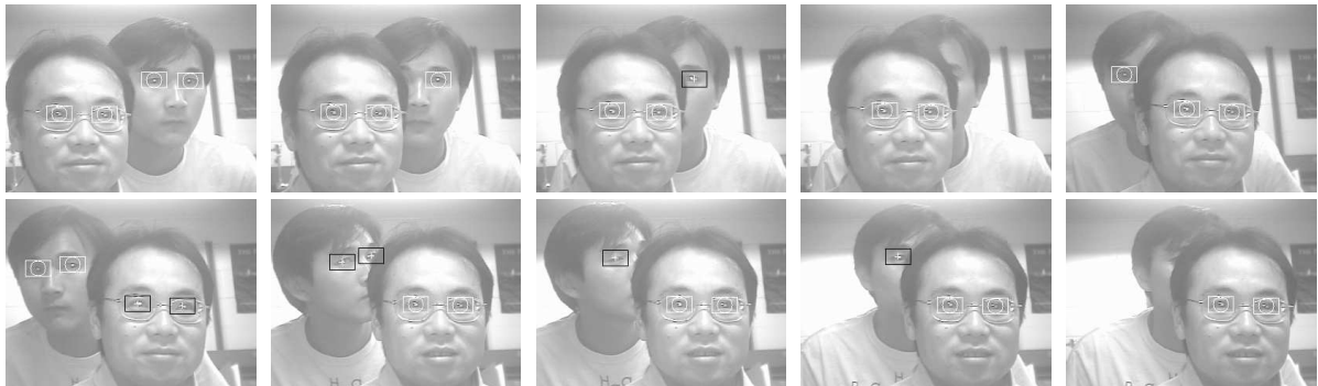
Fig. 26. Tracking results of combined eye tracker for an image sequence involving multiple persons occluding each other's eyes. White rectangles show the eyes tracked by the Kalman tracker while the black rectangles show the eyes tracked by the mean shift tracker.
