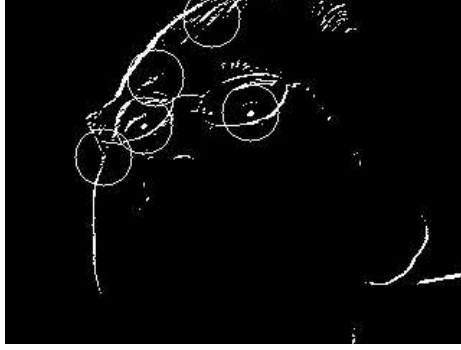
Fig. 8. The thresholded difference image after removing some blobs based on their geometric properties (shape and size). The blobs marked with circles are selected for further consideration.
