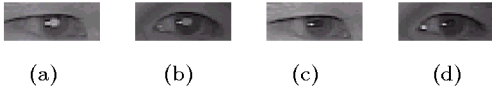
Figure 3. The eye images: (a)(b) left and right bright pupil eyes; (c)(d) corresponding left and right dark pupil eyes
