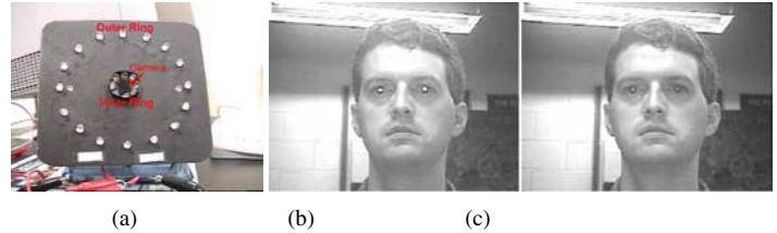
Figure 1. (a) Hardware setup: the camera with an active IR illuminator (b) bright pupils in an even field image (c) dark pupils in an odd field image
