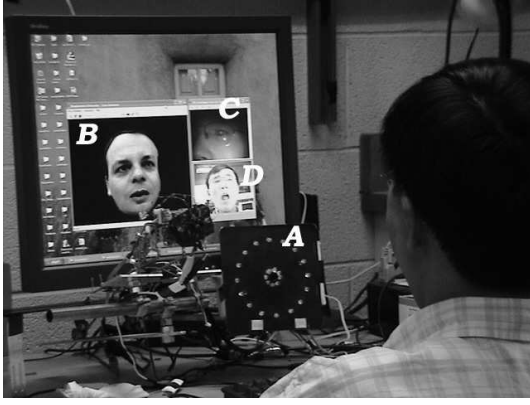
Figure 2: System Setup. A: IR LED rings and IR active camera; B: Animated avata; C: Tracked pupil; D: Tracked face in video
