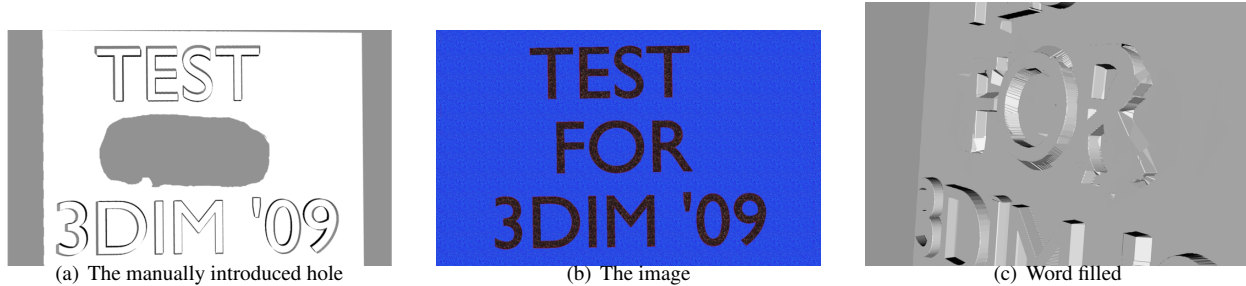
Figure 8. Letters experiment. (a) Scan of letters with middle “FOR” removed to create a hole. (b) Corresponding image. (c) Inpainted geometry.
