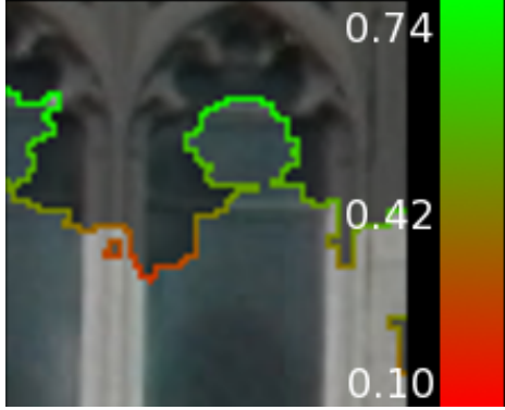
Figure 5. Fill-in order, expressed on a scale from red (low priority) to green (high priority).
