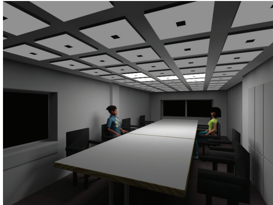
Figure 14: The configuration for Experiment 3, an example of non-uniform, occupancy-dependent lighting.
