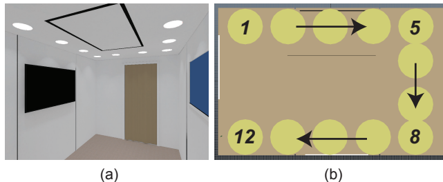
Figure 17: The configuration of Experiment 4. (a) Smart Space Testbed simulation with lighting from LED fixtures. (b) Diagram of the room from above indicating fixture layout.
