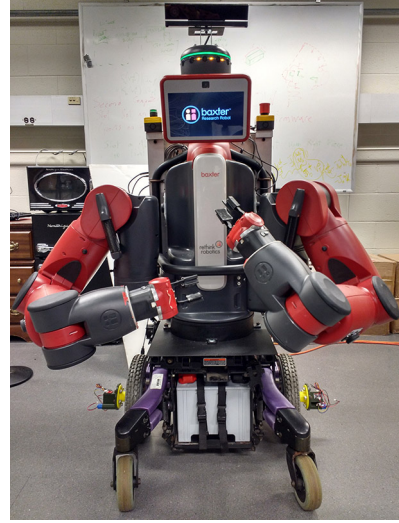
Fig. 3. The Baxter-On-Wheels (BOW). The robot has two 7-degree of freedom arms and a nonholonomic wheelchair base. An RGB-d sensor is mounted on the head for a downward-facing view of the cloth.
