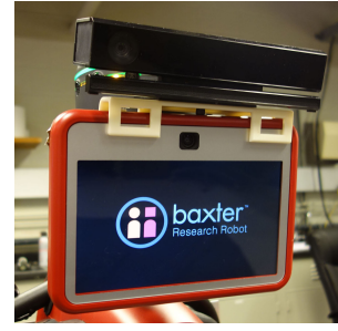
Fig. 2. Microsoft Kinect mounted on Baxter's facescreen.
