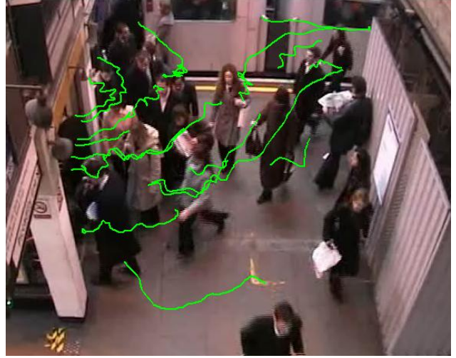
Fig. 3. Some of the longest point tracks extracted from a crowd scene video. The point tracks are overlaid on one of the frames from the video sequence.
