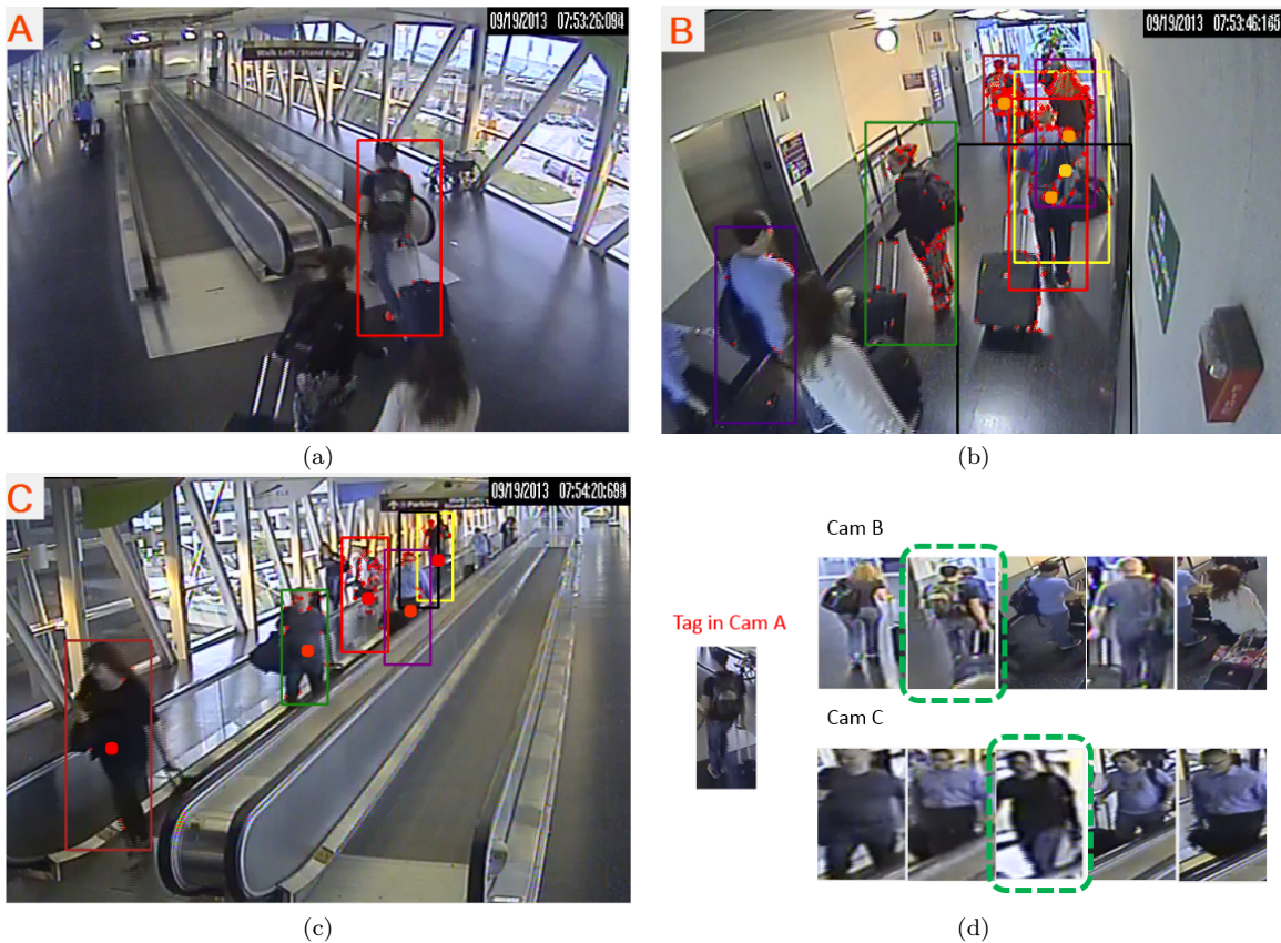
Figure 5: Sample results from the airport human re-identification system. (a) Tagging the person of interest in camera A, (b) Tracking in camera B, (c) Tracking in camera C, (d) Re-identification results (green boxes indicate correct candidates).
