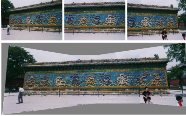
Fig. 5. Images from a non-translating camera, composed into the same frame of reference by appropriate projective transformations.
