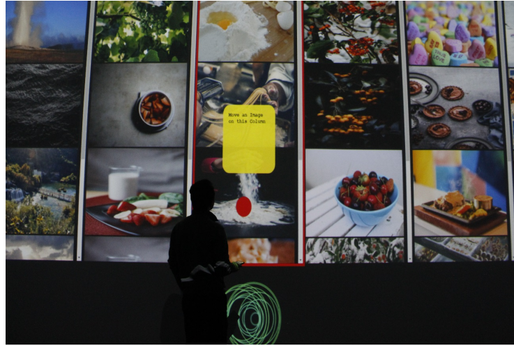
Fig. 4: Experiment 1 setup. The red dot (appearing next to the silhouette of the user) acts as a cursor to interact with the spatially selected column. The yellow text box, shown in the column that the user is interacting with, directs user tasks, in this case “Move an image from this column.”
