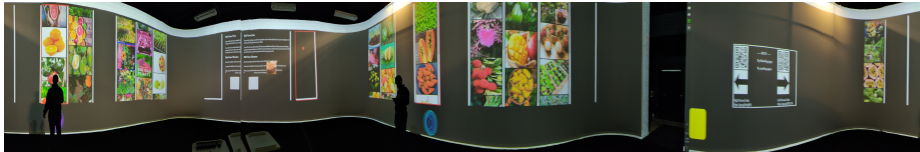
Fig. 1: Multiple users simultaneously interacting with a large screen using their smartphones and voices, coupled with spatial information about their physical locations. This panoramic image shows a 5m tall 360-degree display wall with a 44m perimeter. Please refer to the video hosted at https://youtu.be/CYqXKyHTO_U for detailed interaction examples.
