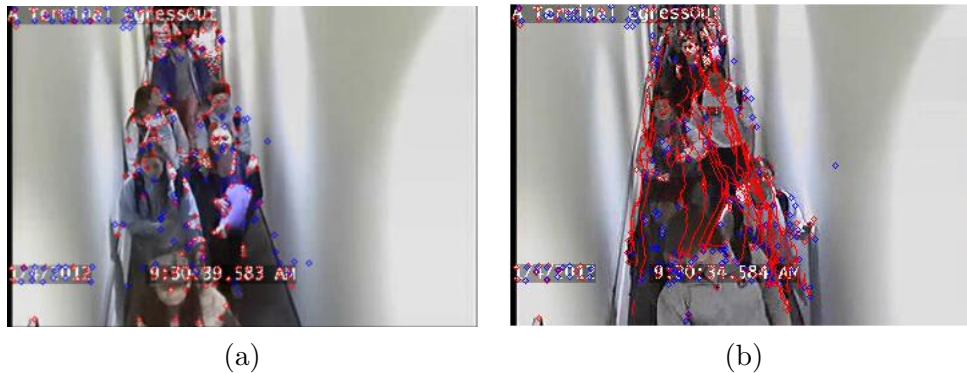
Figure 1: Results of feature tracking. (a) Features detected in the image. (b) Point tracks extracted from a video sequence.
