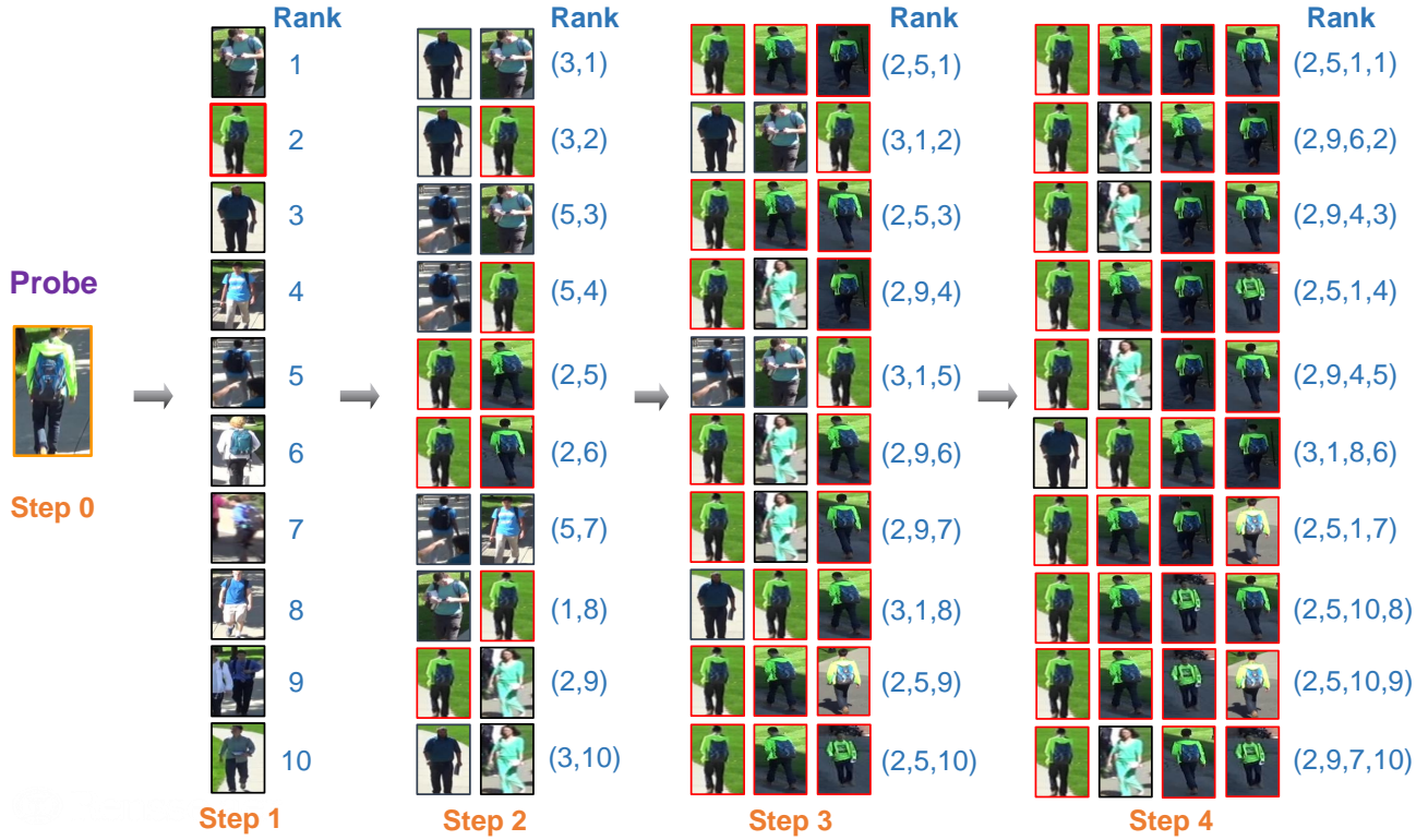
Fig. 6: A visualization of the top-10 retained reappearance sequences from step 1 through 4 for one experimental probe. At each step i , the rank sequences for each candidate along the trajectory are indicated. Red boxes around candidates indicate correct matches. In this case, the ground-truth trajectory for this probe is detected at rank 1 at step 4. Several other trajectories without false alarms (but missing intermediate reappearances) also appear in the top-10 list.
