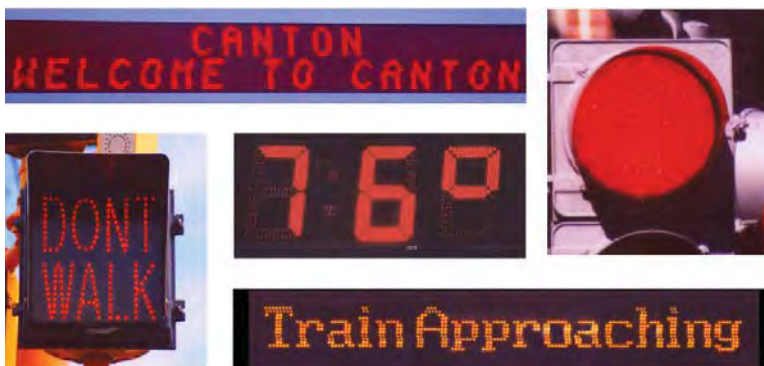
Fig. 1.12. Example of red and amber AlGaInP / GaAs LEDs used in signage applications.
