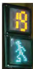
Fig. 1.17. Pedestrian sign indicating number of seconds left to cross street located in Taipei, Taiwan.
