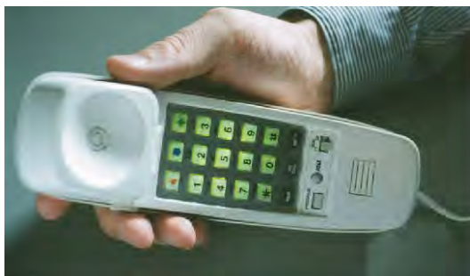
Fig. 1.7. AT&T telephone set ("Trimline" model) with the dial pad illuminated by two green N-doped GaP LEDs. The illuminated dial pad was one of the first applications of green GaP:N LEDs.
