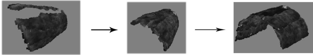
Figure 6.6: Combining point clouds from 3 different views of the phantom.
