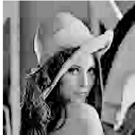
(b) JPEG2000 with a tile size 64 × 64 pixels. Bit rate is 0.1bpp. PSNR=25.12dB.
