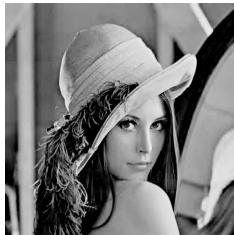
(d) JPEG2000 with a tile size 64 × 64 pixels. Bit rate is 0.5bpp. PSNR=35.67dB.
