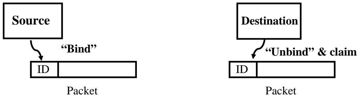
Figure 2: Indirection Prototype: Decoupled Entities (Source, Destination), State (ID in header) and Bind/Unbind Operations
