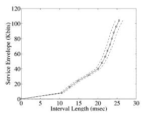
Fig. 4. Service envelope for multiplexed on-off sources.
