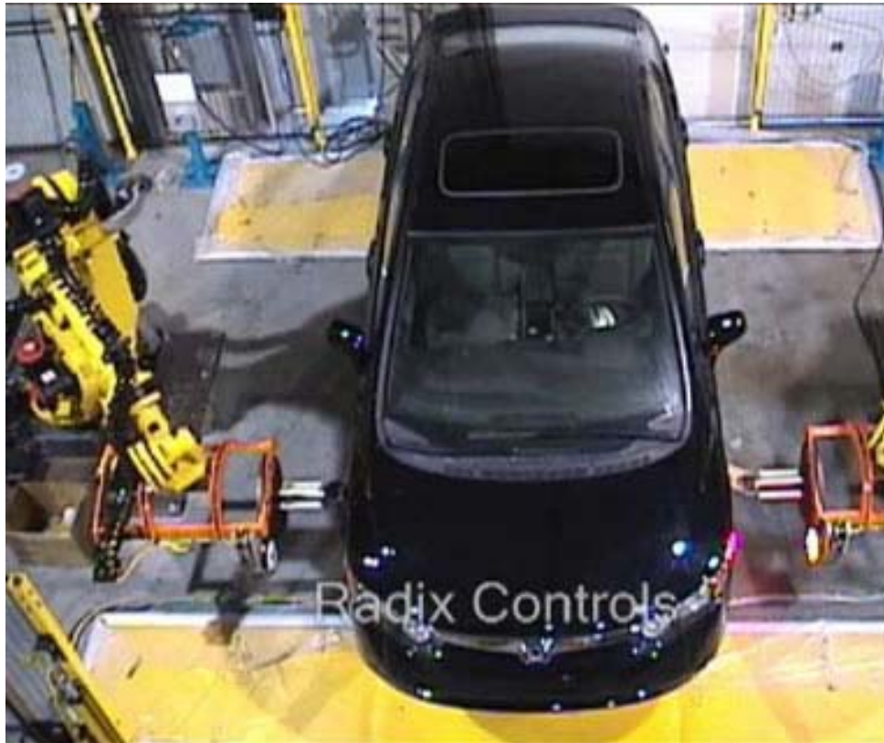
Vision-guided robots position nut runners on wheels
