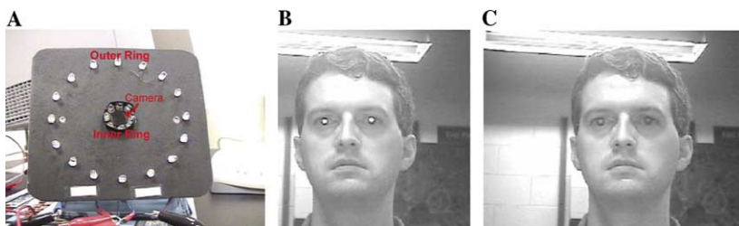
Fig. 2. (A) Hardware setup: the camera with an active IR illuminator (B) bright pupils with even field image (C) dark pupils with odd field image.
