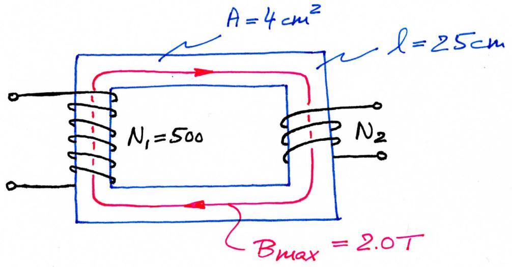
$$B_{\text{max}} = B_{\text{residual}} = 2.0 \text{ T} = 2.0 \text{ Vs/m}^2$$
