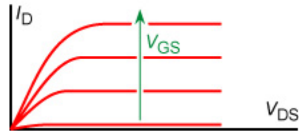
Saturated velocity model: g_m is independent of V_{GS}
