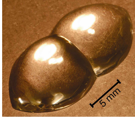
Fig. 3. Photograph of a polarization-enhancing encapsulation shape
