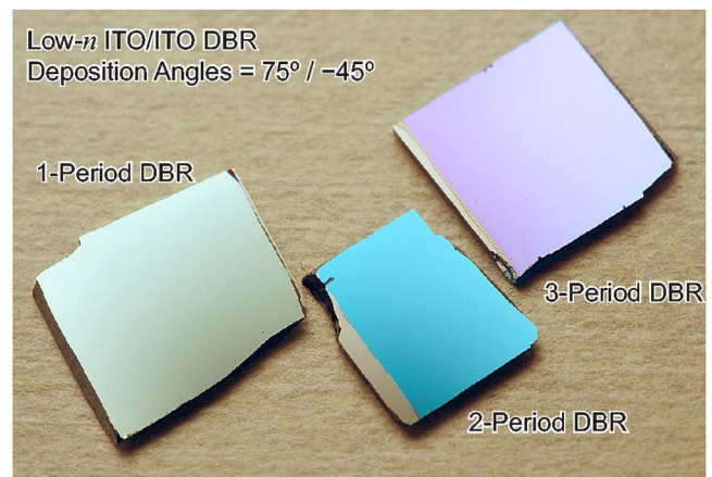
FIG. 4. (Color online) Optical micrograph of one-, two-, and three-period DBR samples. The two- and three-period DBRs have a bluish color, which indicates higher reflectivity in that wavelength range.
