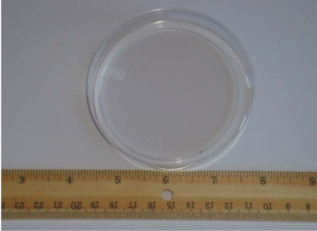
Figure 9: Optical photograph of a nanostructured antireflection coating on a 3-inch glass substrate.
