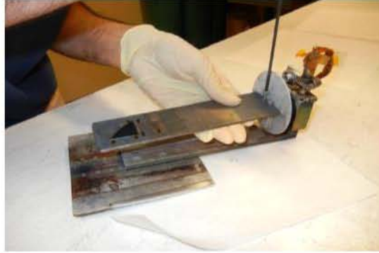
Figure 6.4. Cleaned sample holder and loading of the sample for nanostructure AR- Coating fabrication.
