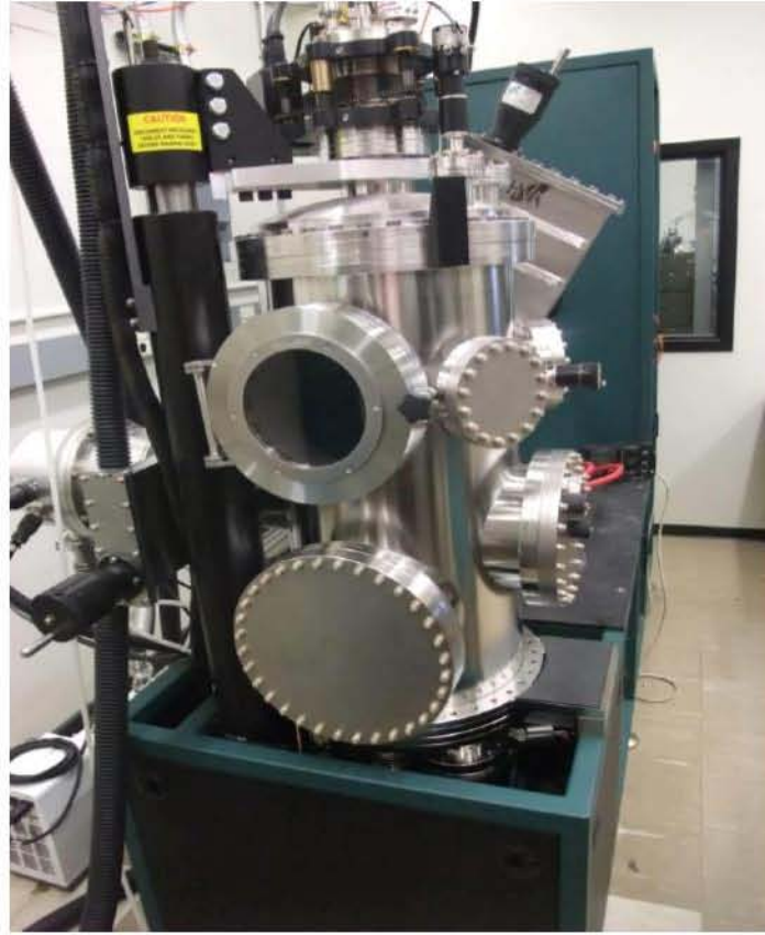
Figure 7.1. E-beam system with modifications for large area nanostructured anti-reflection layer deposition.
