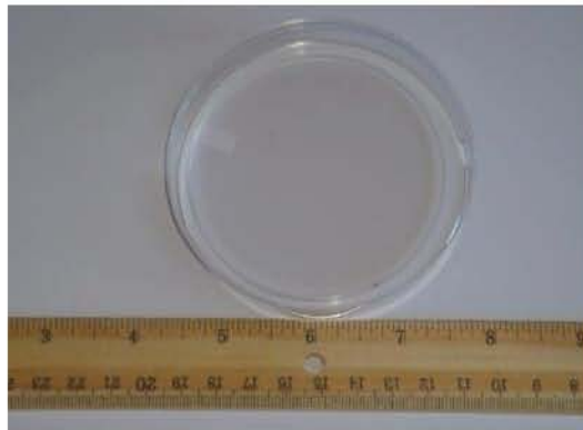
Figure 6.5. Optical photograph of a nanostructured antireflection coating on a 3-inch glass substrate.
