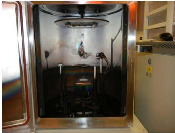
Figure 6.2. Inside view of the Oblique Angle Nanostructure AR Coating Chamber.
