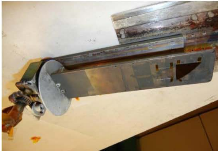
Figure 6.3. Enlarged view of the Nanostructure AR Coating sample holder.
