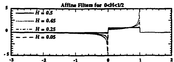
Continuous time wavelet filters associated with the fractional Brownian motion for 0 < H < 1/2 .
