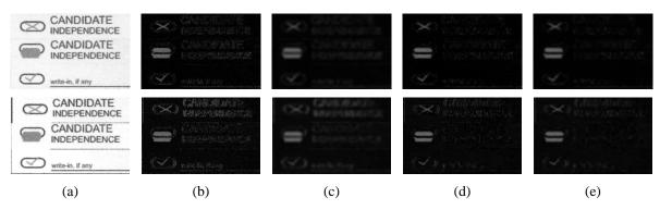
Figure 2: (a) samples from original image, (b)-(e) corresponding samples when differenced with methods D1-D4. Top row is for dark scanned original, bottom row is for light scanned original. Black is no image difference.
