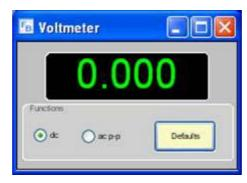
The meter is simply an ac and dc voltmeter that displays the value in digital form. It can be used in ac mode by clicking ac p-p, in which case the value represents the peak to peak value. If the waveform has a high crest factor the results can be slightly surprising. In dc mode, if there is an ac component present, the average value is displayed.
