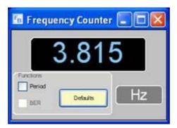
This has the facilities of a conventional frequency meter/counter. It will display in either frequency or time. If the input amplitude is too low a warning message will be displayed.
