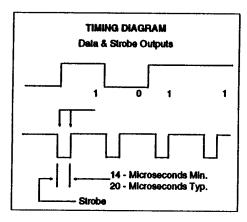
output in a serial bit-by-bit format. Each bit is represented by a data output level and a strobe. The level at this output represents the decoded data, where a high zero bit.
