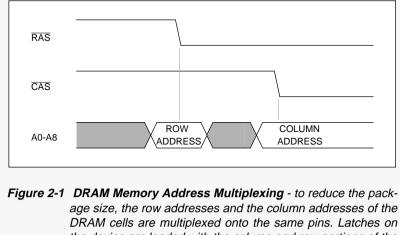
age size, the row addresses and the column addresses of the DRAM cells are multiplexed onto the same pins. Latches on the device are loaded with the column and row portions of the address by the signals Column Address Strobe (CAS) and Row Address Strobe (RAS).
