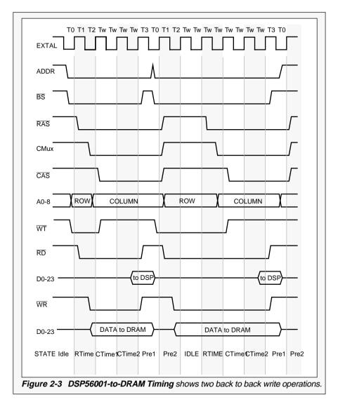
**NOTE:** Figure 2-3 shows the timing relationship between the DSP56001 Port A and a DRAM module. The Port A interface is described in Section 1.2 DSP56001 Memory I/0 Basics.
