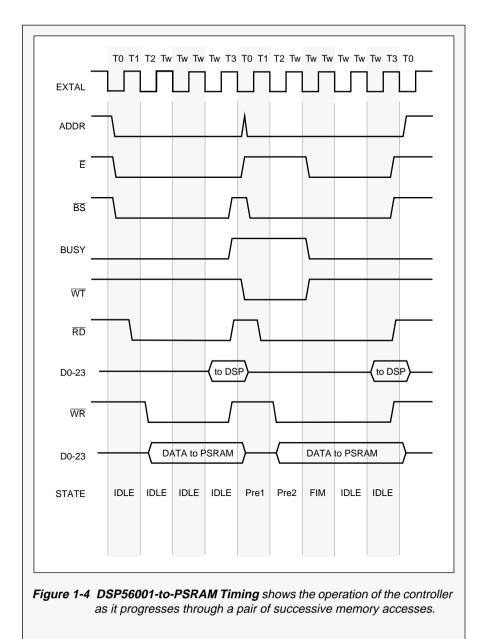
The timing diagram in Figure 1-4 shows the operation
