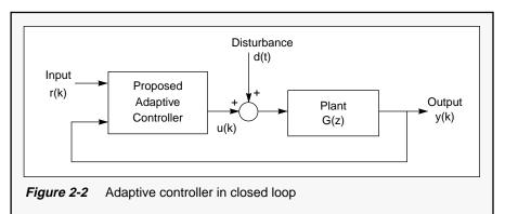
This system will be used to measure the performance of the adaptive controller as it works to maintain (or equal) the desired response in the presence of a disturbance.
