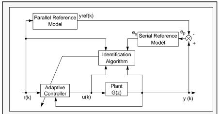
Figure 3-1 Adaptive control using reference models in closed loop
