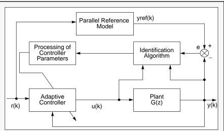
Figure 3-2 Generalized predictive control using closed loop
