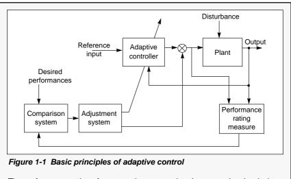
The performance rating of a system is measured and compared to the design goal. The adaptive system modifies the parameters of the adaptive controller in order to maintain the performance rating close to the desired value.
