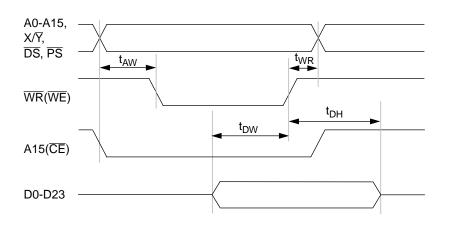
Figure 2-3 Write Cycle Timing Diagram
