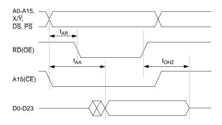
Figure 2-2 Read Cycle Timing Diagram
