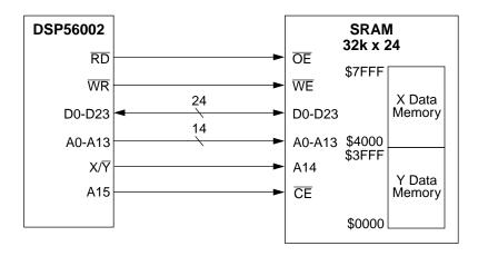
Figure 2-1 DSP56002 Interface to External SRAM
