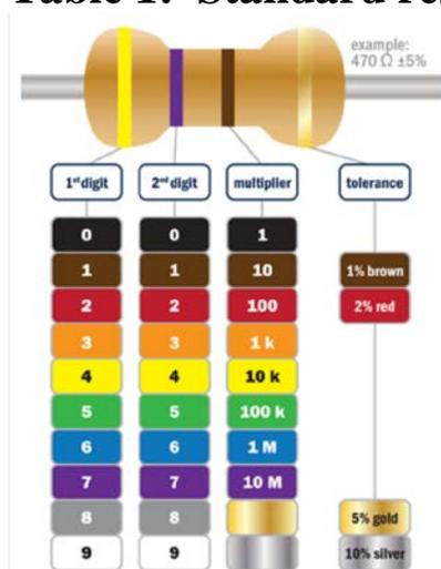
**Figure 1: Resistor color and Tolerance bands**
