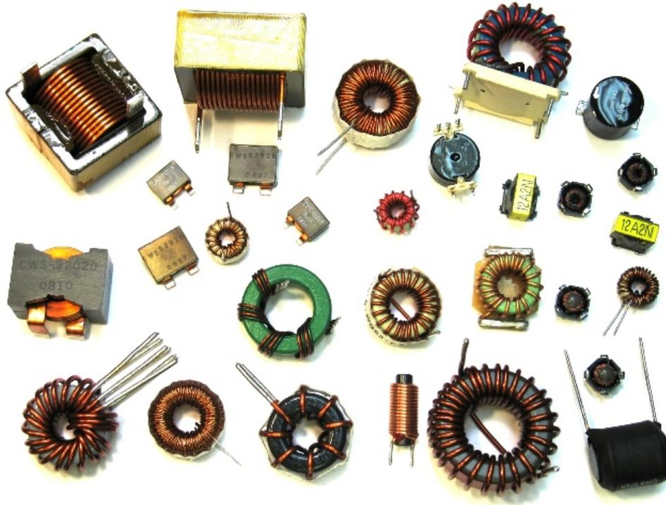
Ideally,  $L = \frac{(\mu_0 N^2 h_c)}{2\pi} \ln\left(\frac{b}{a}\right)$  Henries when the core is air or plastic. Otherwise replace  $\mu_0$  with  $\mu$  for the core material.  $h_c$  is the height of the core material.  $a$  and  $b$  are inner and outer radii and are shown in the figure at the right.
