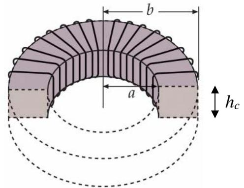
*Calculating Resistance:* When one makes an inductor, the wires used can have a large variety of cross sectional areas. There are some inductors made with very thick wires, while others are made with very thin wires. Thin wires permit one to wind many more turns of wire around a core and thus increase the inductance. Thick wires have lower resistance for any given length. All wires have a resistance given
