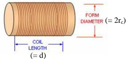
where  $\mu_0 = 4\pi \times 10^{-7}$  Henries/meter. If the core is not air, but rather some magnetic material, replace  $\mu_0$  with  $\mu$  which is usually many times larger than  $\mu_0$ . By many times we can mean as much as  $10^5$  times larger. You should know that this formula only works well when the length  $d$  is much, much larger than the radius  $r_c$ .
