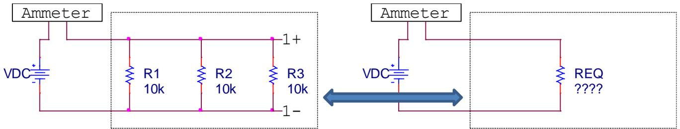
Resistors in parallel are another basic circuit configuration. Again, referring to the section at the beginning of the laboratory, you can determine the equivalent resistance. Once again, use the Ammeter and Voltmeter to experimentally find the equivalent resistance. How does your measurement compare to the calculated value?
