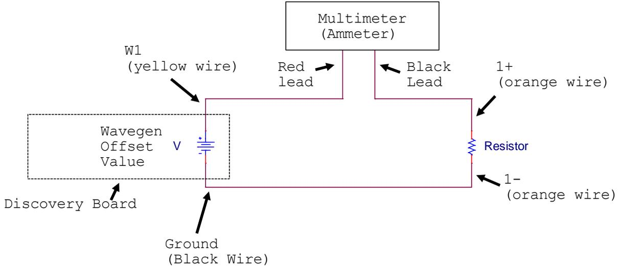
Measure the voltage across and the current through the resistor, as described below.
