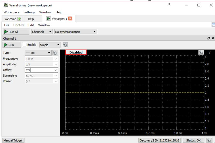
**Note:** Depending on your software installation, the red wire ( $V^+$ ) can also be used as a variable DC source. You can see if that option is available by clicking the Supplies tab on the Welcome tab.
