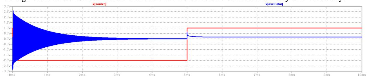
Clearly, the decaying oscillation is too fast to be observed using the time scale above, so the scale was expanded to show 2µs/Div during the time from 30µs to 50µs Use the information in plots to answer the following:
