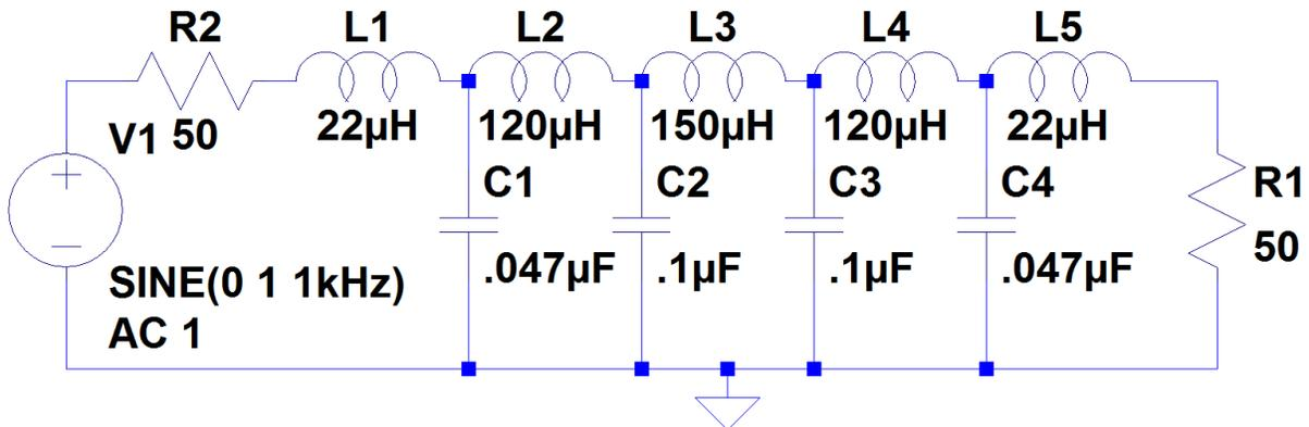
The filter shown above is a good approximation to what is known as a Butterworth Filter. The components were chosen from commercially available inductances and capacitances to be close to the ideal values found using Butterworth's analysis. This circuit diagram is used to build the circuit, not simulate it because it does not include all necessary ideal components.
