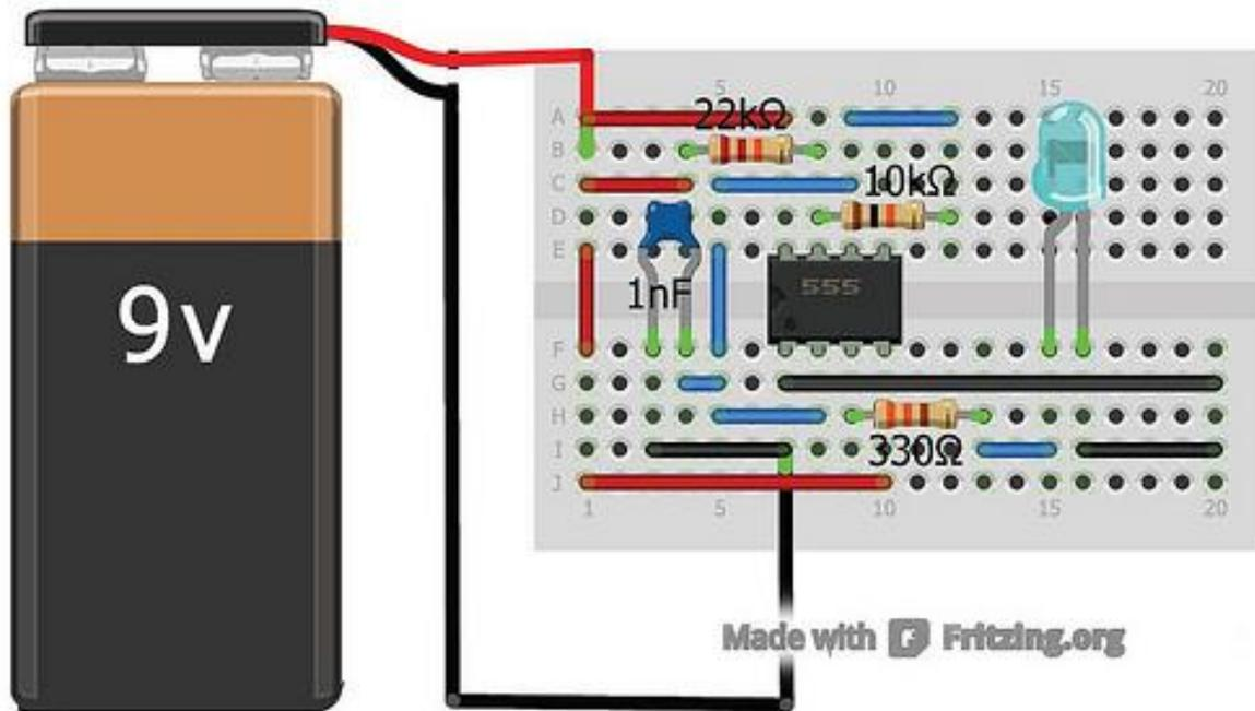
On a 555 Timer chip, what pin do we connect to for the output voltage? That is, where do we connect the load? *Circle the correct answer. Hint: You may have already been told this.*
