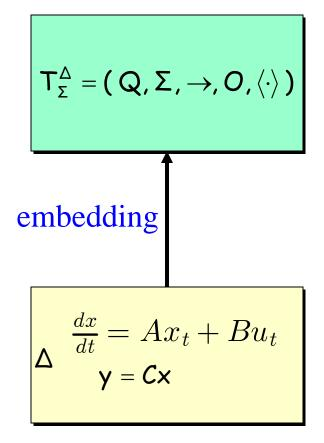
Transition System  $T_{R}^{\Delta}$ State set  $Q = X = R^n$ Label set  $\Sigma = R_{\perp}$ Observation set  $O = Y = R^{p}$ Linear Observation Map  $\langle x \rangle = Cx$ Transition Relation  $\rightarrow \subseteq X \times R_{\downarrow} \times X$ ∃u<sub>[0,†]</sub> with  $x_{1} \xrightarrow{\dagger} x_{2} \Leftrightarrow x_{2} = e^{At}x_{1} + \int e^{A(t-s)}Bu(s)ds$
