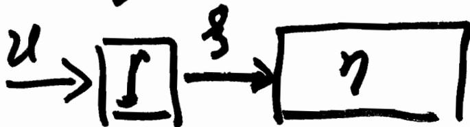
Backstepping : Design a "virtual" control for  $\eta$ -subsystem, backstep it over the integrator to design "u".
