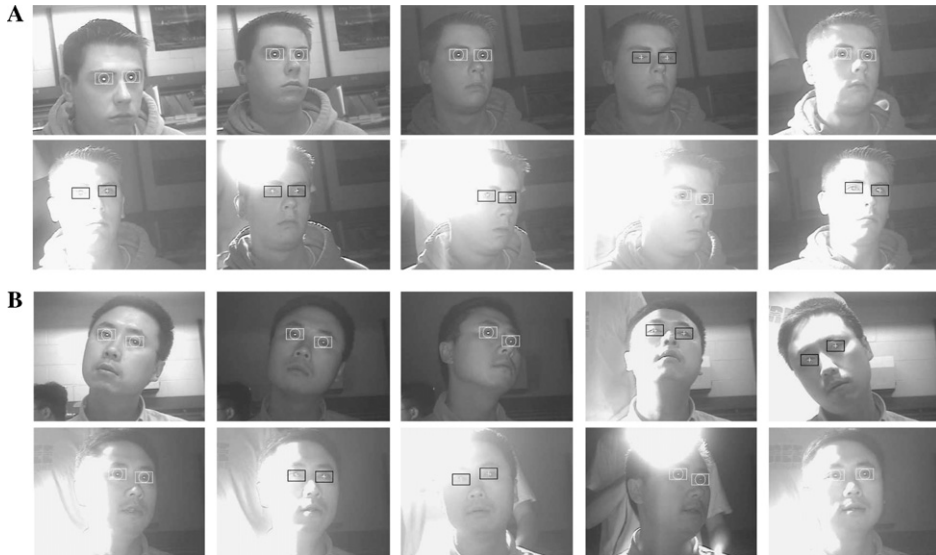
Fig. 23. Tracking results of the combined eye tracker for two image sequences (A) and (B) under significant illumination changes. White rectangles show the eyes tracked by the Kalman tracker while the black rectangles show the eyes tracked by the mean shift tracker.
