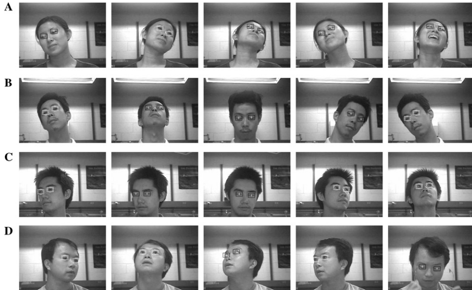
Fig. 22. Tracking results of the combined eye tracker for four image sequences (A), (B), (C), and (D) under significant head pose changes. White rectangles show the eyes tracked by the Kalman tracker while the black rectangles show the eyes tracked by the mean shift tracker.
