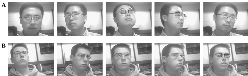
Fig. 24. Tracking results of the combined eye tracker for two image sequences (A,B) with persons wearing glasses. White rectangles show the eyes tracked by the Kalman tracker while the black rectangles show the eyes tracked by the mean shift tracker.
