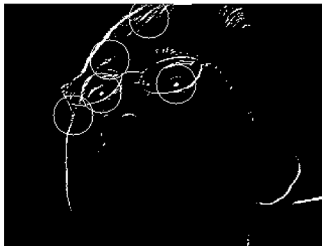
Fig. 8. The thresholded difference image after removing some blobs based on their geometric properties (shape and size). The blobs marked with circles are selected for further consideration.
