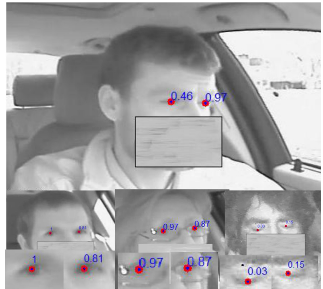
Fig. 7. Samples of eye detection and eye state estimation results on extreme challenging SHRP2 driving database. The faces of the subjects are partially covered as this identity information can not be made public under the terms of a data sharing agreement.
