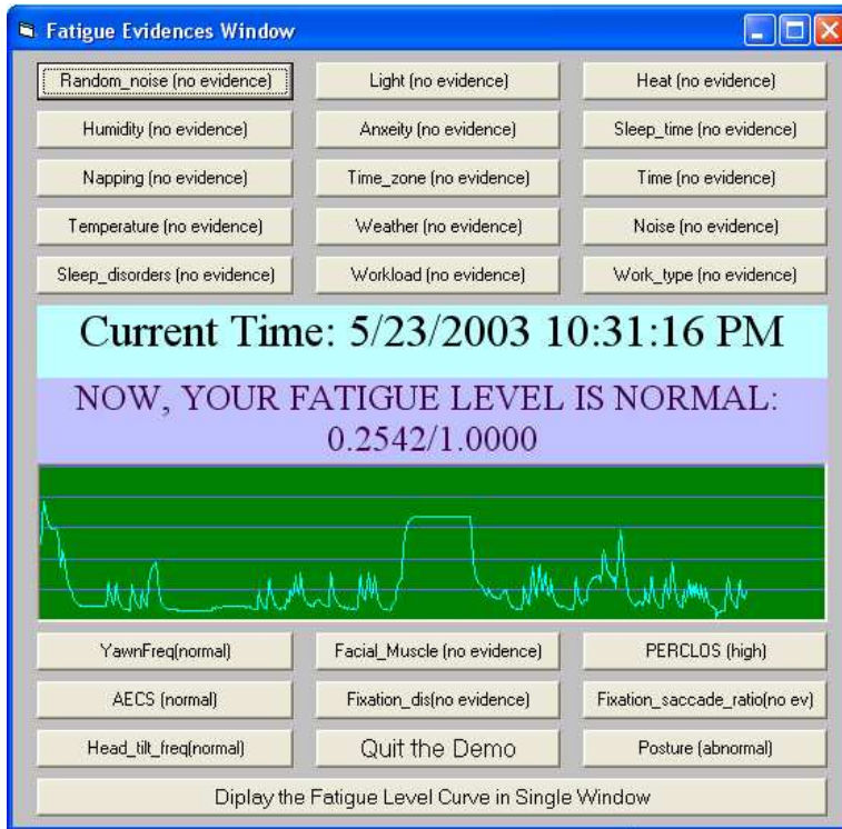
Fig. 23. The visual interface program panel. It displays the composite fatigue score over time.
