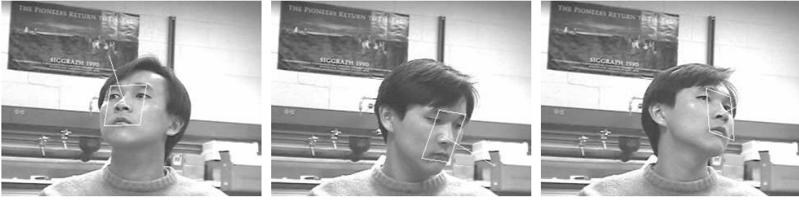
Fig. 12. Face and face pose tracking results for images randomly selected from one video sequence. The white rectangle indicates the tracked face region and the white line represents the normal of the face plane, which is drawn according to the estimated face pose.
