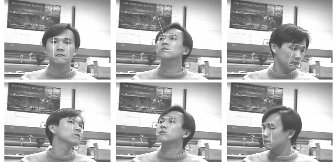
Figure 5. Face pose tracking results taken from one video experimental sequence, which are randomly selected. The white rectangle indicates the tracked face region and the white line is the norm of the face plane which is drawn according to those three angles.
