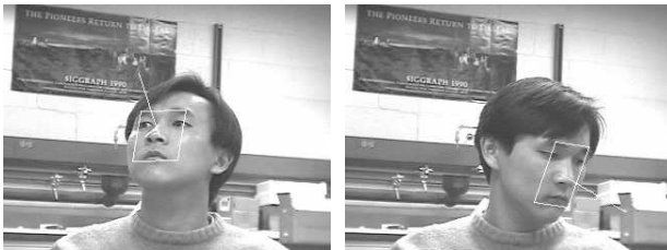
Fig. 5. Face pose tracking results for images randomly selected from one video sequence. The white rectangle indicates the tracked face region and the white line represents the normal of the face plane, which is drawn according to the estimated face pose.
