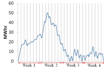
Fig. 3. Storage levels in MWhr when a 1MW windfarm and ESS with unlimited capacity are operated using a linear program to achieve upper bound revenues for Case 1, ( $d = 1\text{MW}$ ,  $\eta = 1$ ).
