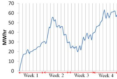
Fig. 6. Storage levels in MWhr when a 1MW windfarm and ESS with unlimited capacity are operated using ETP for Case 3 i.e., using imperfect statistics, ( $d = 1\text{MW}$ ,  $\eta = 1$ ).
