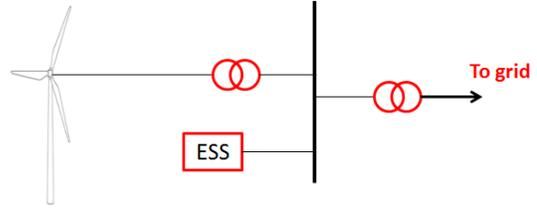
Fig. 1. Windfarm and ESS system.
