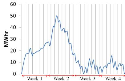
Fig. 5. Storage levels in MWhr when a 1MW windfarm and ESS with unlimited capacity are operated using a linear program to achieve upper bound revenues for Case 2, ( $d = 1\text{MW}$ ,  $\eta = 0.9$ ).
