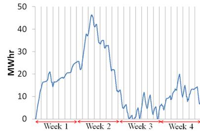
Fig. 4. Storage levels in MWhr when a 1MW windfarm and ESS with unlimited capacity are operated using ETP for Case 2, ( $d = 1\text{MW}$ ,  $\eta = 0.9$ ).
