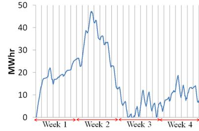
Fig. 2. Storage levels in MWhr when a 1MW windfarm and ESS with unlimited capacity are operated using ETP for Case 1, ( $d = 1\text{MW}$ ,  $\eta = 1$ ).
