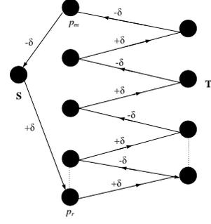
Fig. 10. A cycle that improves total value (revenue) of the flow (energy allocation).
