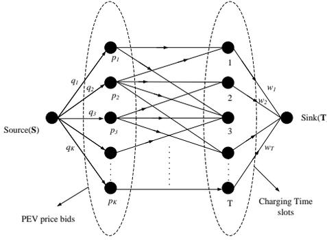
Fig. 5. Network flow representation of the optimal charging problem.
