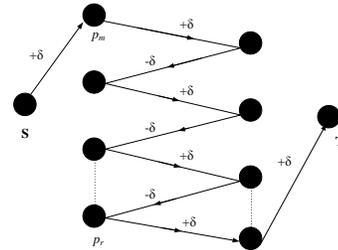
Fig. 9. An augmenting path in the residual flow graph of  $f$ .
