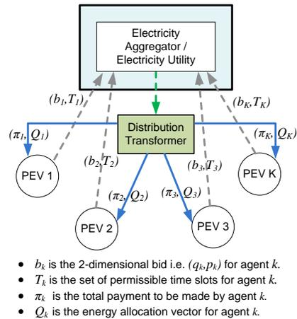
Fig. 4. Schematic diagram of the PSP auction process.
