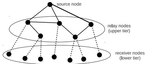
Figure 2: Streaming video delivery in the 2-tier network model. Figure 3: Graph representation of the 2-tier network model in Figure 2.
