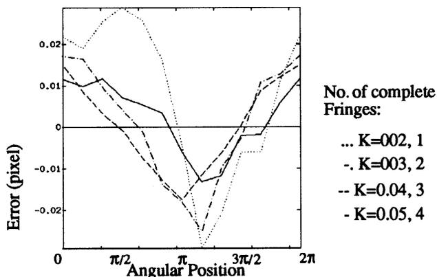
Fig. 14. Error as a function of the number of complete fringes used in the optimization when the image is corrupted with Gaussian noise.  $\varphi = 0$ , test image of  $640 \times 480$  pixels, Gaussian noise  $\sigma = 5$ , center at (320, 240), true center at  $\rho = 0.1$  pixel.
