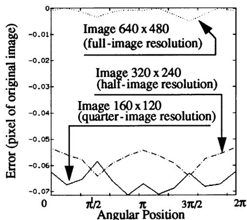
Fig. 17. Error of the center location for three different image resolutions (measured in pixels of the original image). True center at  $\rho = 0.1$  pixel.
