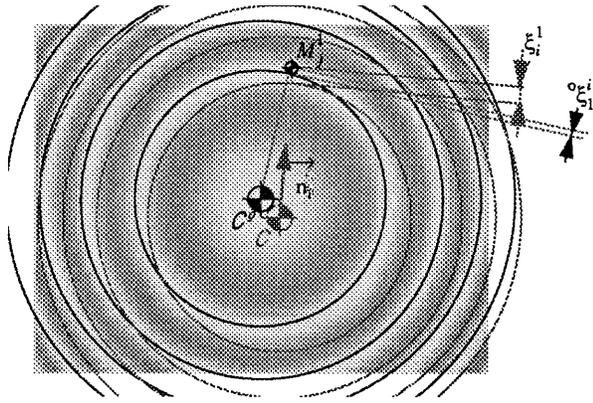
Fig. 4. Perturbation on four concentric fringes. This brings the successive radii in compliance with Eq. (3) and minimizes the total least-squares sum of normal errors.
