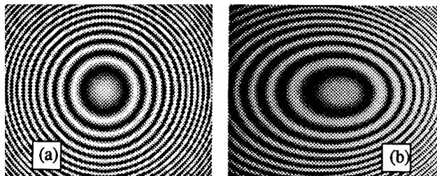
Fig. 20. Simulation of the effect on the captured fringe pattern when angular defects occur between the reference-mirror plane and the camera plane: (a) No angular defect—the pattern is circular concentric. (b) Angular defect of  $45^\circ$  about the vertical axis—the pattern is no longer circular.
