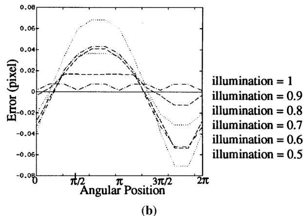
Fig. 18. (a) Illumination function across the fringe pattern. (b) Error on the center location when different levels of illumination are applied to the image.  $\varphi = 0$ , test image of  $640 \times 480$  pixels, noise-free center at  $(320, 240)$ , true center at  $\rho = 0.1$  pixel.
