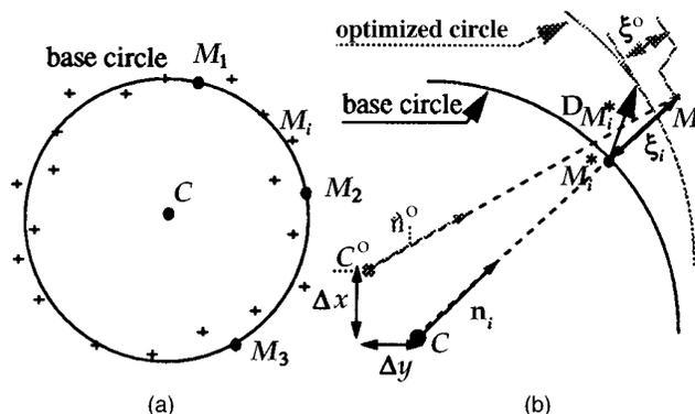
Fig. 3. Optimization by use of perturbations of a circle: (a) Three points defining a circle called the base circle. (b) Optimization of the base circle by variation of the center location and radius.
