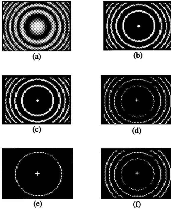
Fig. 5. Procedure for center-location determination: (a) Computer-generated image. (b) Peak extraction. (c) Fringe labeling. (d) Fringe skeletonizing. (e) Approximate center computation on the fringe with the maximum number of points. (f) Final optimization with four consecutive fringes.
