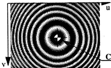
Fig. 2. Sample circular zone plate pattern produced by the interferometer shown in Fig. 1. The two-dimensional position of the center  $C$  is the measurement parameter.
