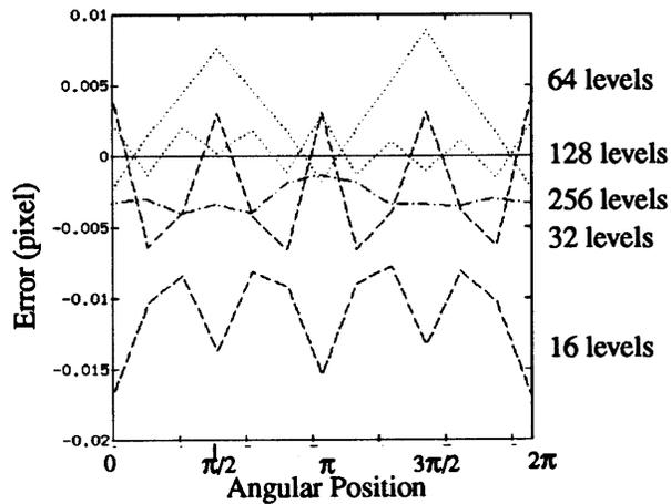
Fig. 19. Error on the center location when different levels of quantization are applied to the image.  $K = 0.03$ ,  $\varphi = 0$ , test image of  $640 \times 480$  pixels, noise-free center at (320, 240), true center at  $\rho = 0.1$  pixel.
