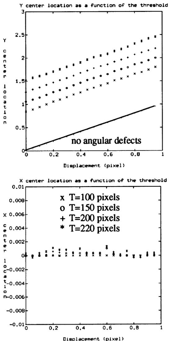
Fig. 22. Simulation of a theoretical image of the effect of detector-plane angular defects on the center location for different thresholds  $T$ .
