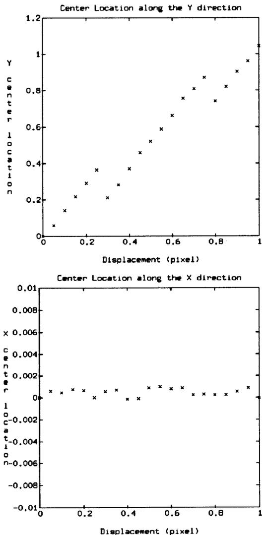
Fig. 21. Center location along the principal directions for an angular defect about the vertical direction equal to  $0.05$  rad and the direction of displacement rotated by  $0.1$  rad about the horizontal direction for a computer-generated image.
