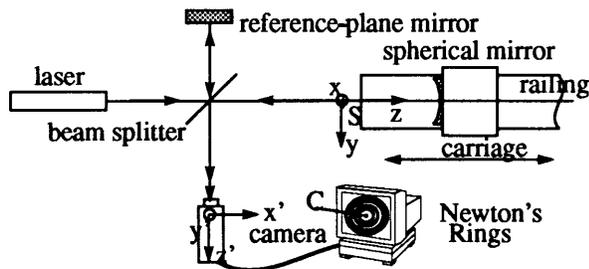
Fig. 1. Interferometer for translational error measurements.
