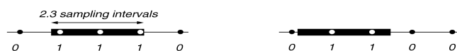
Fig. 4. Sampling a black stroke 2.3 sampling-intervals long may yield a bitmap of three or two black pixels.
